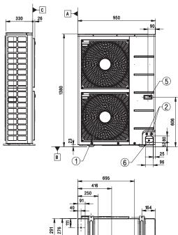
5-I.D.  $\emptyset$  20 holes for drain connection
