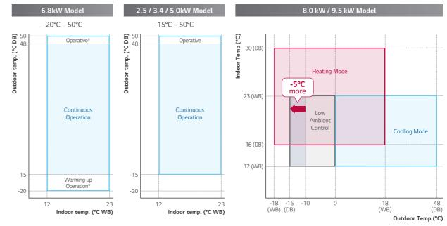
\* Warming up operation and operative means that the outdoor unit operates to reach the range of continuous operating, however it may not operate continuously due to safety or protection logic.
